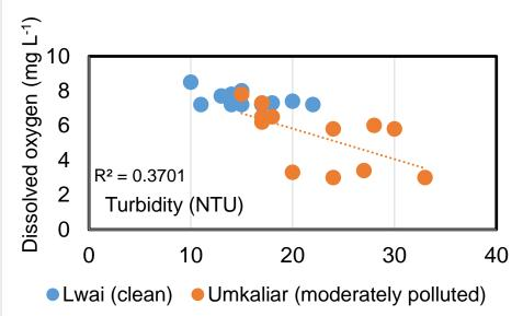
Figure 3. Upper panel shows that the temperature was a significantly important variable in determining DO in moderately polluted stream, while in Lwai stream DO stayed stable across the year. Lower panel also depicts that turbidity explains a significant trend in DO values in moderately polluted stream, while in Lwai stream the pattern is non-significant.
