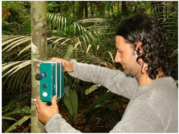
Photo2: Placing the autonomous ultrasound recorder in the sampling plot inside an island.
