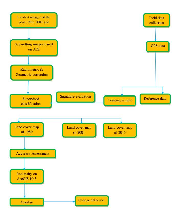
Figure 4:Methodology for LULC change detection.
