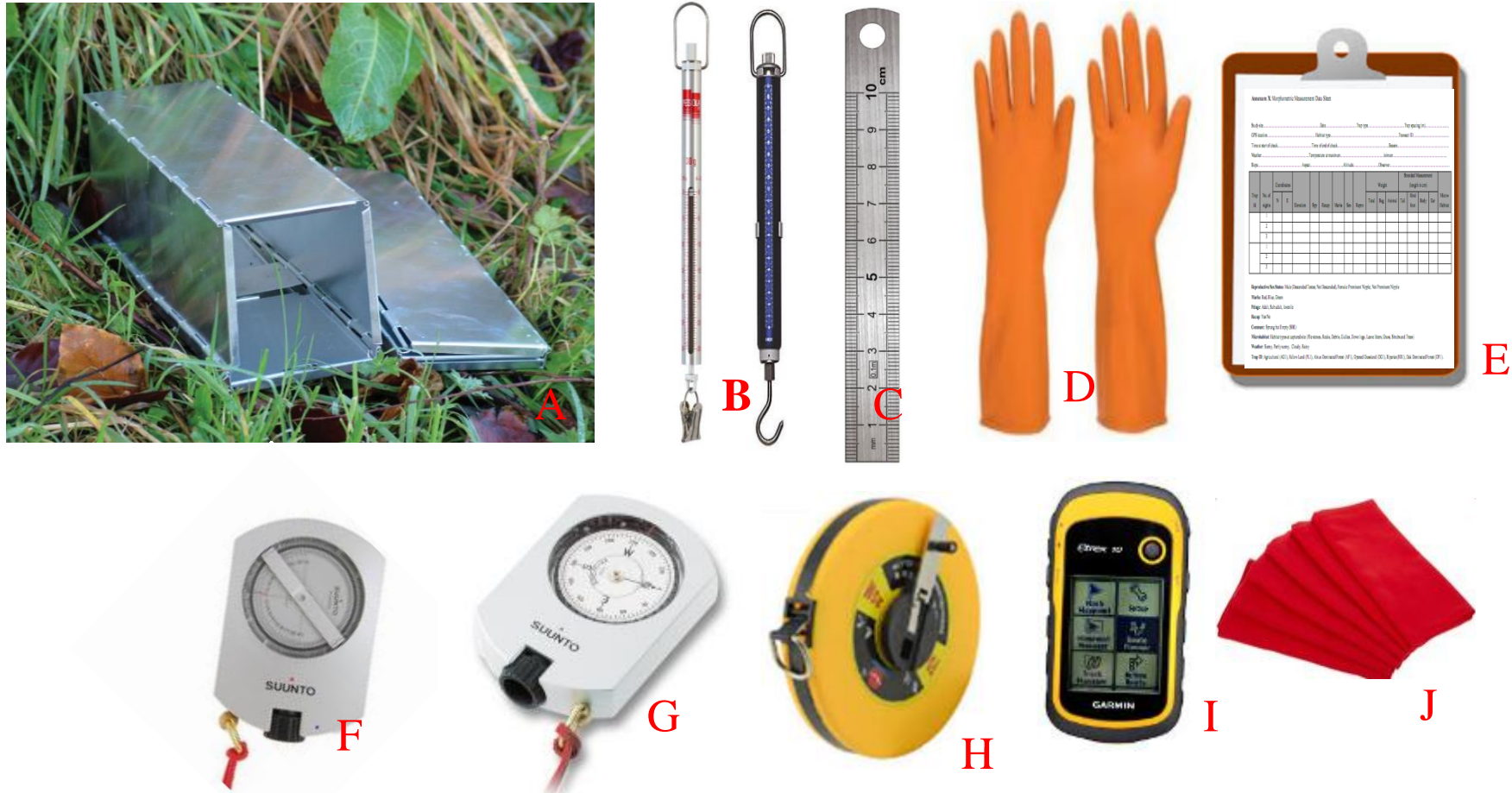
Figure 6. (A) Sherman trap, (B) Pesola spring balance, (C) Stainless ruler, (D) Glove, (E) Data sheet, (F) Clinometer, (G) Compass, (H) Measuring tape, (I) GPS, (J) Flagging cloth
