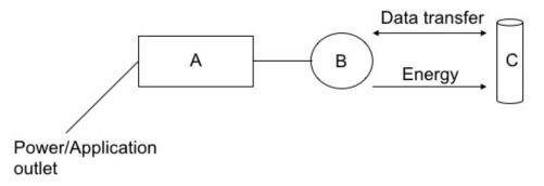
**Figure 2.1:** The main components of an RFID system are the reader (A), with an attached antenna (B) and the tag (C).
