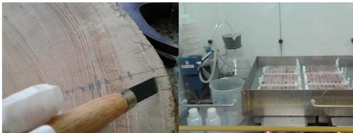
Left: Selection of tree rings, previously dated, for flake extraction. Right: Cellulose extraction from Cedrela odorata samples.
