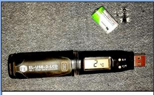
Figure 1. EL-USB-2-LCD, Climatic data logger
