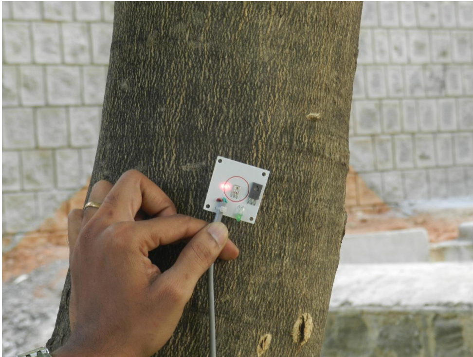
Fig. 9 & 10: LASER transmitter (top) receiver (bottom) units testing at day light. At complete darkness the unit is working for a range around 50 meters but with surrounding light the range is getting reduced and at twilight the system is working up to 30 meters.
