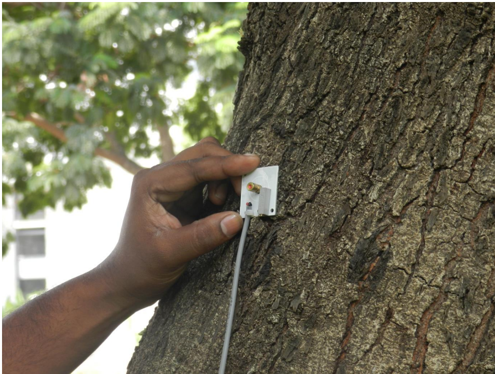
Fig. 8: Outdoor experimentation of designed LASER transmitter and receiver unit at BIT.
