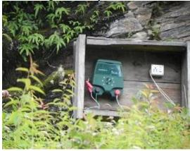
Pic 7. Energizer that regulates the flow of current in electric fence.
