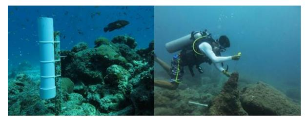
Left: A sediment trap deployed at one of the study sites. Right: Saw Darrick from DIVEIndia deploying a light data logger.
