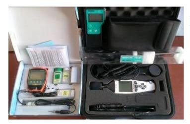
For microclimatic measurements in field conditions I bought next technical equipment: a) soil moisture meter Rixen M-700S (1 pcs.); b) soil pH and temperature meter Ezodo MP-103S (1 pcs.); c) environment multimeter Flus ET-965 (1 pcs.). This equipment will allows getting clear data about air temperature, air humidity, illumination, soil moisture, soil temperature, and soil pH in localities of investigated *Aconitum* taxa.
