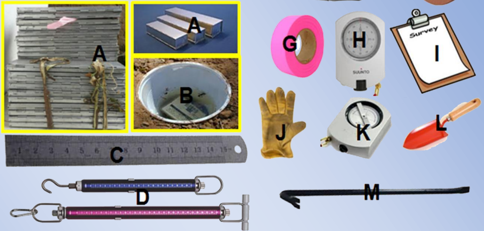
Figure 4: A. Sherman traps; B. Pitfall traps; C. Ruler; D. Pesola Spring; E. GPS; F. Measuring tape; G. Ribbon; H. Compass; I. Datasheet; J. Gloves; K. Clinometer; L. Scoops; and M. Crowbar
