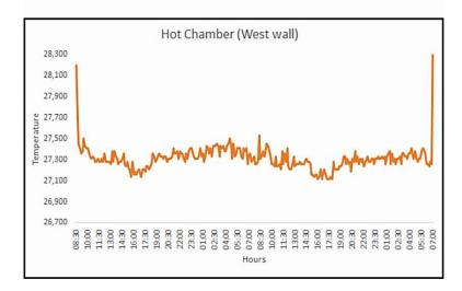
Figure 3.Temperature and relative humidity profiles from 2 main galleries within La Barca Cave, Guanahacabibes, Pinar del Rio, Cuba. Peak temperatures observed at the beginning in some graphs correspond to the moment in which data-loggers were installed.
