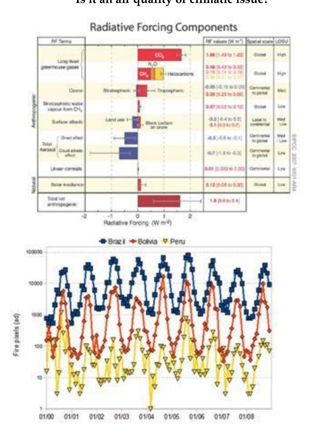
**Fig. 1.** Fire pixels from NOAA satellites for 2000 to 2008 (from DSA/INPE) over Peru, Brazil and Bolivia. There is an important amount of pollution produced by biomass burning mainly in Brazil. Note the logarithmic scale of Y axis.
