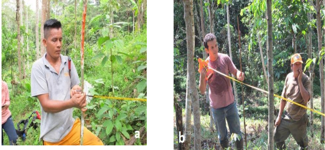
Figure 6: Placing a peg in the centre of the sub plot (a) and measuring the area boundary (b). (Photo: Valeria Saldaña).
