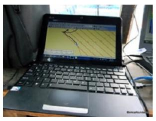
Laptop connected with GPS – showing survey transects and boat orientation
