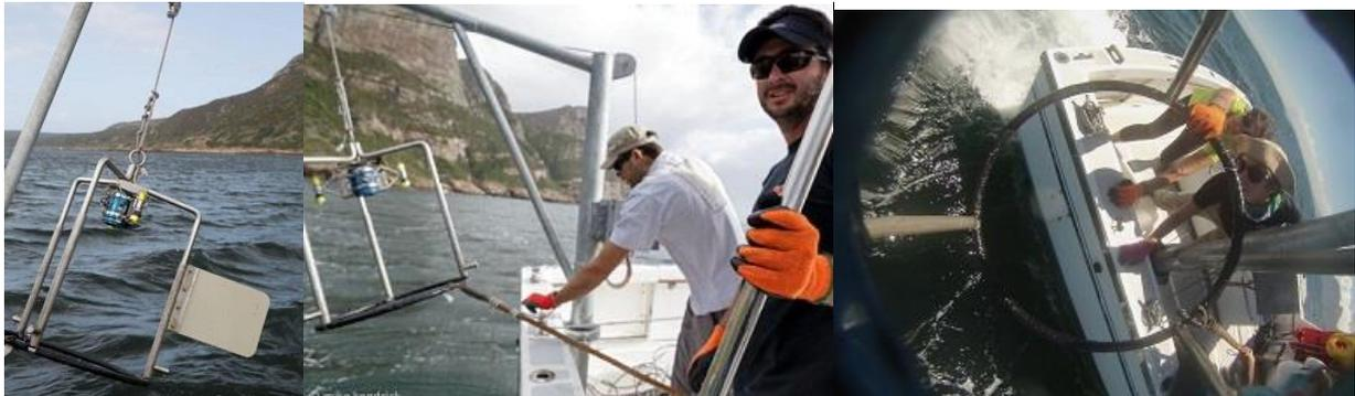
**Left:** Our “jump camera” – a custom-made steel frame with a downward-facing camera to capture images of the seafloor and the invertebrates inhabiting the region. **Middle:** Fieldwork volunteers steady the jump camera between deployments. **Right:** A jump camera selfie – the view from the camera as we check between deployments that all is still operational.
