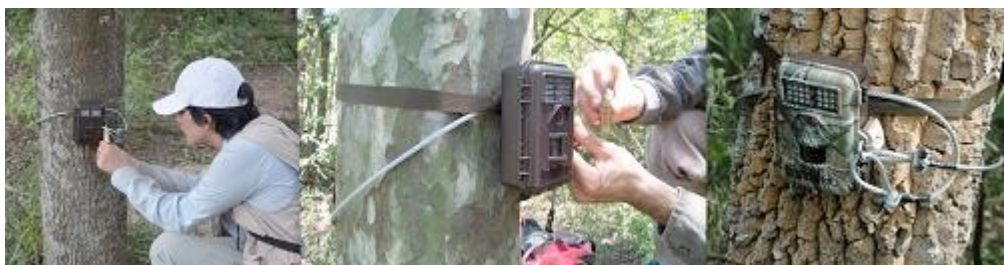
Figure 2. The installation and security arrangement of camera-trap.
