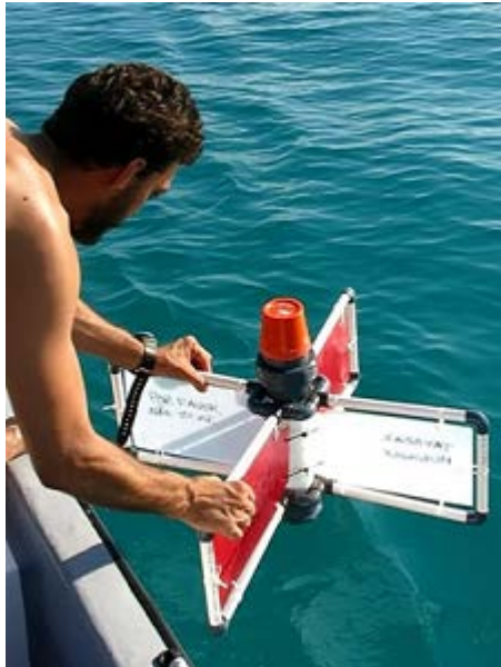
Figure 2 Release of surface drifter for current tracking. The home made drogue is fitted with a GPS transmitter that acquires and sends the drifter coordinates to the user at a set time interval of 10 min.
