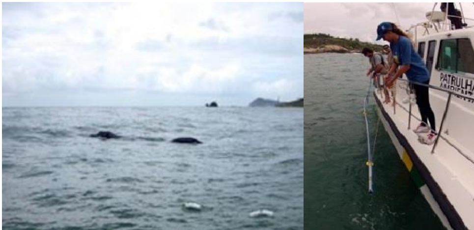
Left: A linear hydrophone array (white buoys) is used to record the sounds of whales (note an individual's head and tail stock behind the buoys). Photo: Paulo A. C. Flores. Right: Deployment of the hydrophone array in the study area. Photo: Karina Groch
