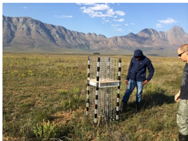
Luvuyo Dlamini (SAEON intern) and Abri de Buys (SAEON technician) test the multi mini-disc non-destructive biomass measurement technique.
