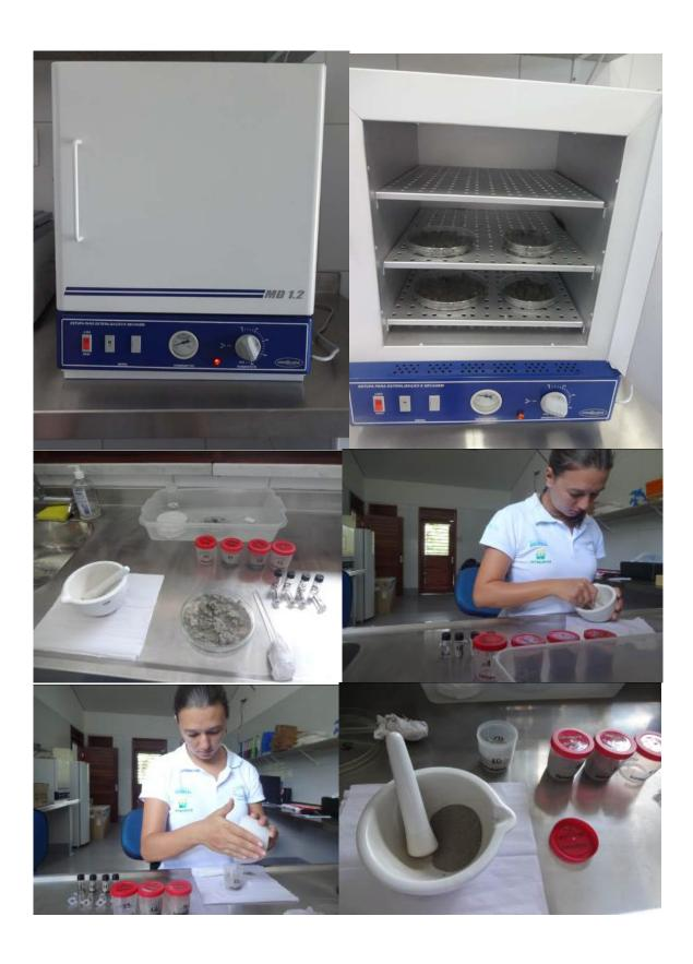
Preparation of the sediment samples collected for the organochlorine analysis
