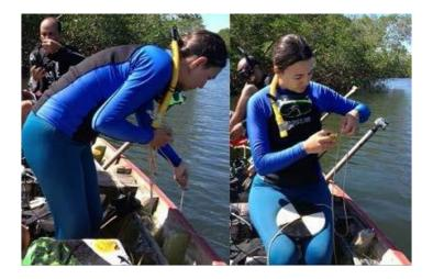
Figure 10. Measurement of water turbidity using Secchi disc.
