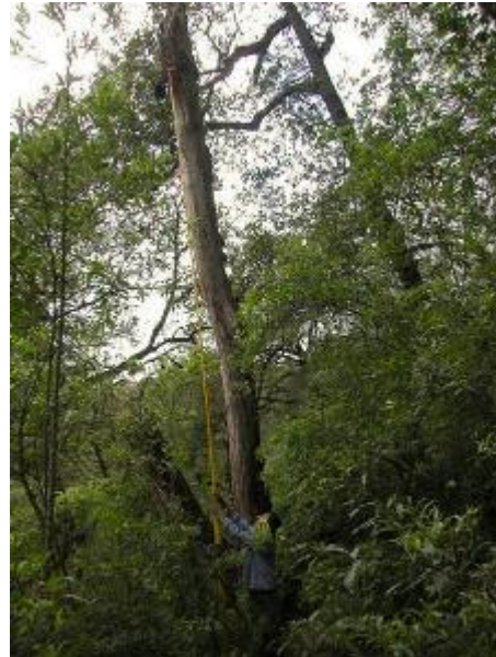
Figure 7. Inspection of cavities with camera system mounted to a 15 m extensible pole.
